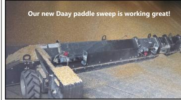
structed last fall. This proves why they are called 'zero entry'.....notice how clean the floor is behind the sweep? No one had pushed a broom on that floor—and no one was in the bin! At Farmers Elevator, we are working to provide a safe and efficient operation for our workers and for you, the patrons we serve. And by the way, in the face of all this rain, we are very glad we are not digging any holes to begin any construction immediately!
